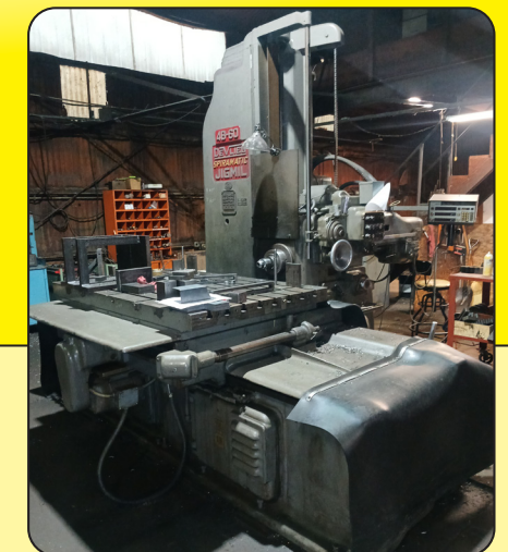
Devlieg Spiramatic Jig Mill
