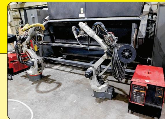
Motoman Robotic Welding System Including Motoman Welding Positioner with (2) Motoman Robots
