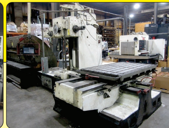
Lucas 441B-72 Horizontal Boring Mill
