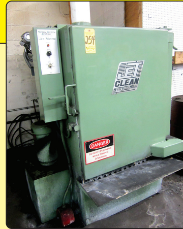
Storm Vulcan Mattoni Electric Heated Jet Master Parts Washer
